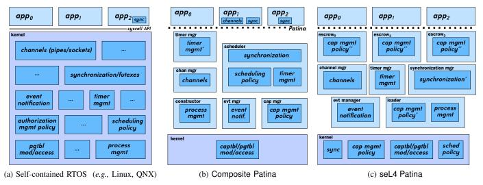
Fig. 1: Differing system structures for an RTOS API. The dotted line is the Patina API, light-blue boxes are protection domains, dark blue are functional modules, and the purple box is the kernel.
